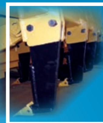
■ RIPPERS Rippers are rear mounted; tines are shear bolt protected to 8 tonnes break-out. Shin guards are standard.
