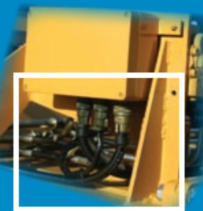
■ CONTROL SYSTEM connects to an external box by common 10 core cable, wired with military-style connectors for extremely reliable performance
