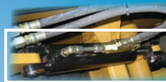
■ CROSS LEVELLER Ram with lock out valve for accurate and reliable control
