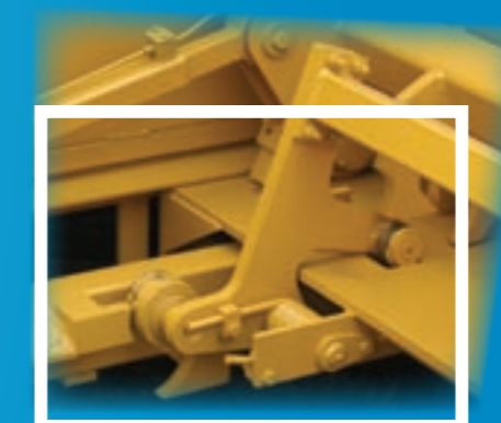
■ EJECTOR AND MOVING FLOOR Patented ejector travels a whole 2.75 metres; running on heavy duty rollers
